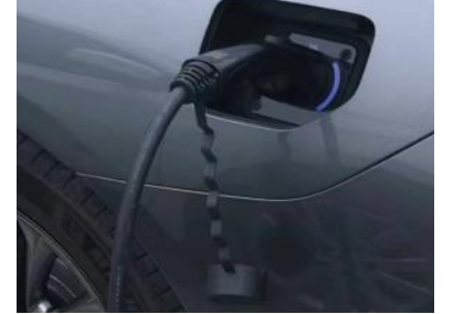
FAW AC vehicle connector with discharging function intergrated
